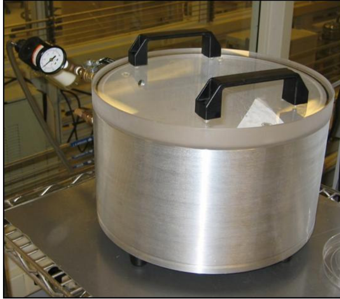
Figure 13. The vacuum chamber used to degas the PDMS mixture.
