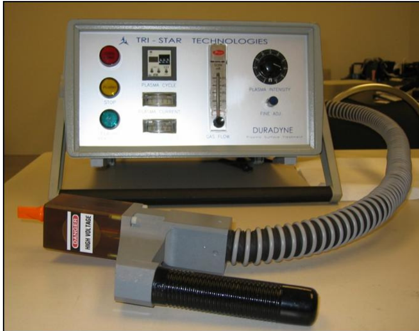
Figure 18. A picture of the plasma bonder and gun used to bond the PDMS devices to glass.
