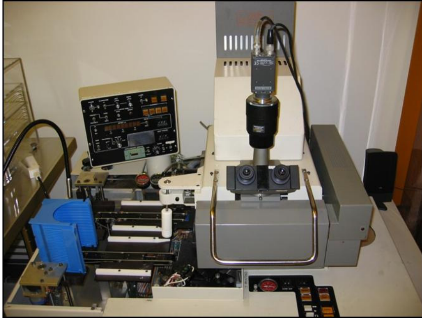
Figure 9. The aligner used for exposure.
