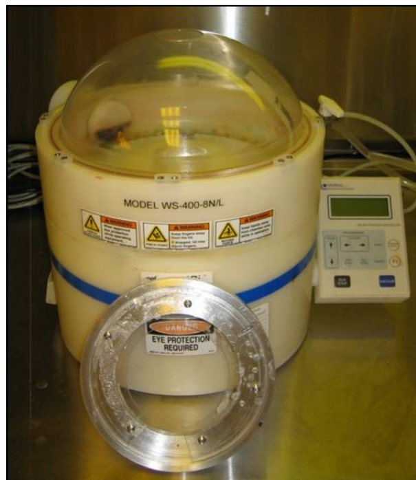
Figure 8. The spin coater used for negative photoresist and centering ring.
