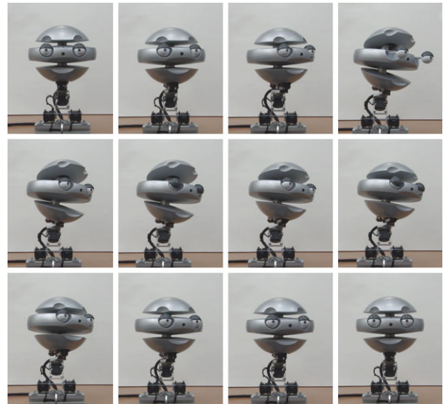
Fig. 4 EMYS: snapshots with movement capabilities
