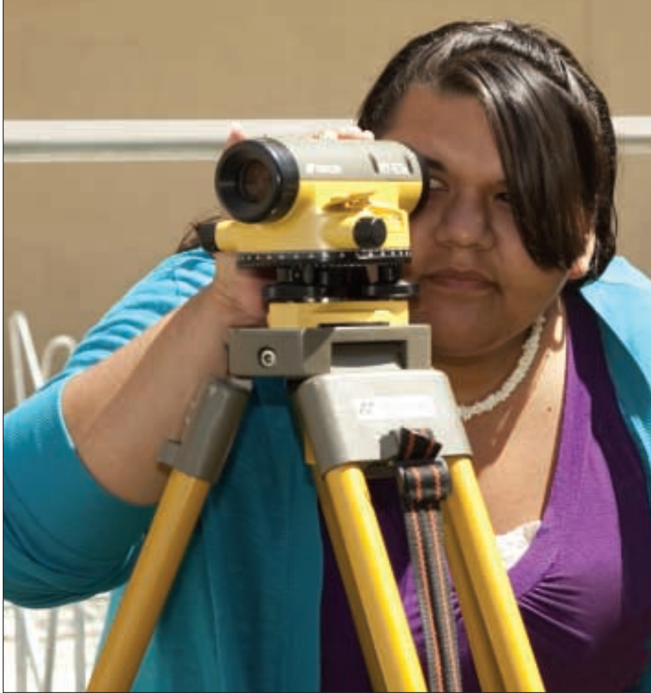
In a surveying exercise, Monica Diaz learns how to operate a construction level (above).
