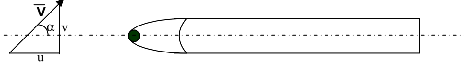
Figure 1. Schematic of Axisymmetric Probe
