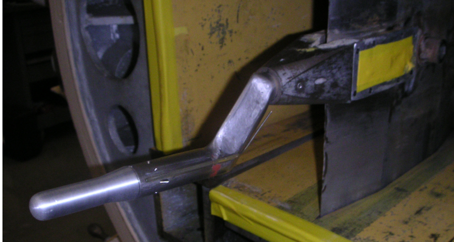
Figure 4. Parabola/Cylinder Probe Mounted in USAFA's Trisonic Wind Tunnel
