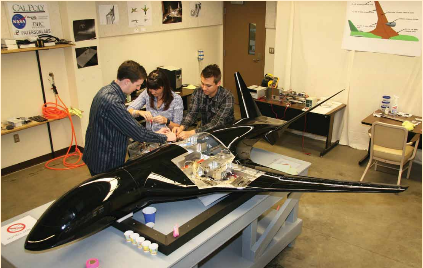
AERO students Eric Paciano and Jonathan Lichtwardt work with professor Tina Jameson, middle, on the AMELIA aircraft model designed for wind tunnel tests.
