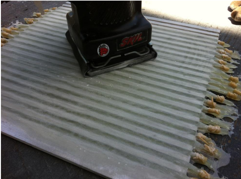
Figure 29. DADs are sanded down until separated from aluminum mold
