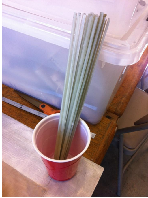
Figure 30. Cured DADs separated from mold
