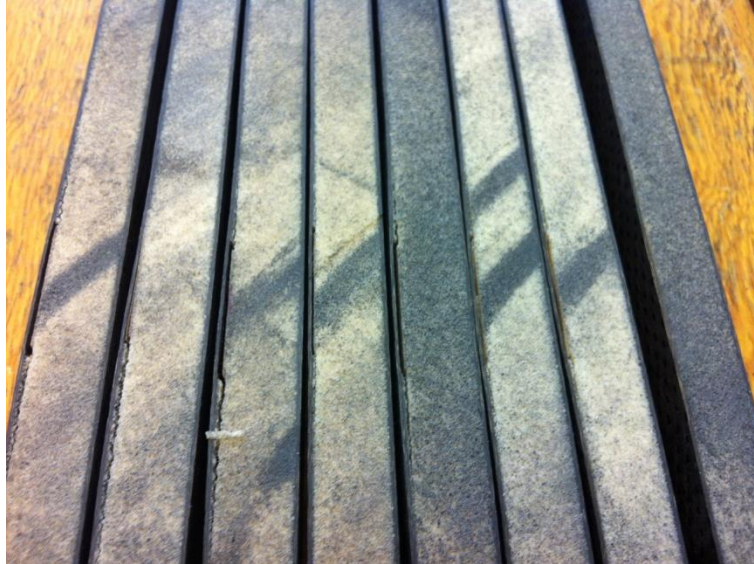
Figure 40. Final failure mode of control beam case with one inch initial delamination.
