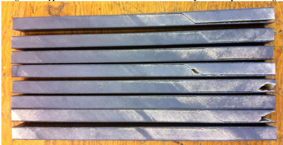
Figure 37. Control case group failure mode nearly identical in each test specimen.
