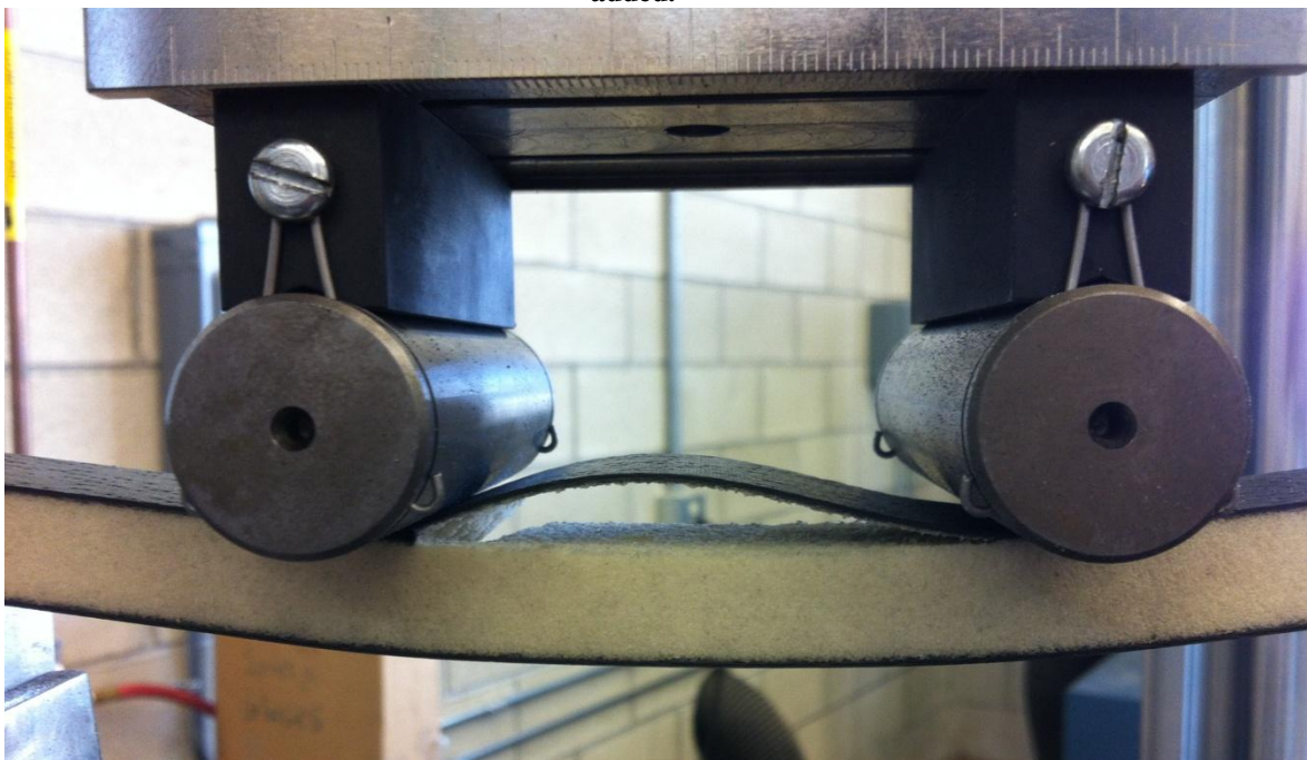
Figure 39. Typical failure mode of initially delaminated control case beams.
