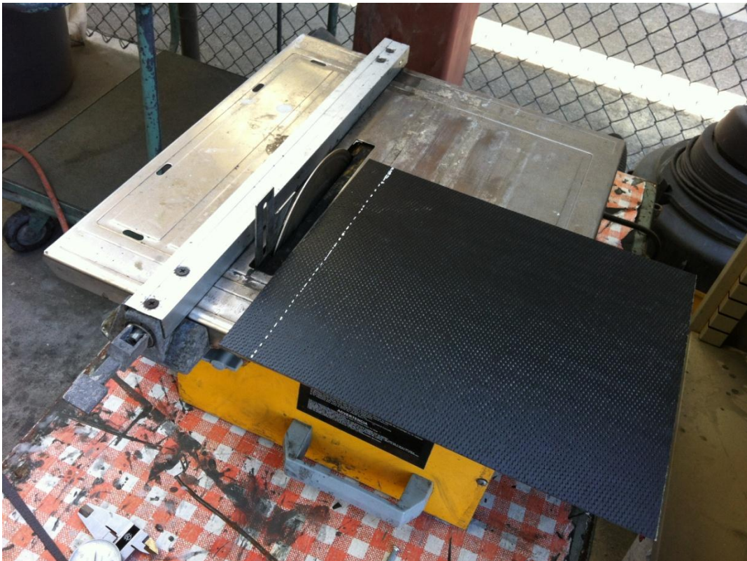
Figure 17. Tile saw used to cut test specimens
