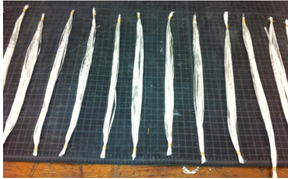
Figure 26. Bundles composed of 15 strands of unidirectional fiberglass
