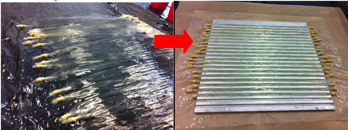
Figure 27. Hand Lay-up Method Used to Fabricate DAD Keys
