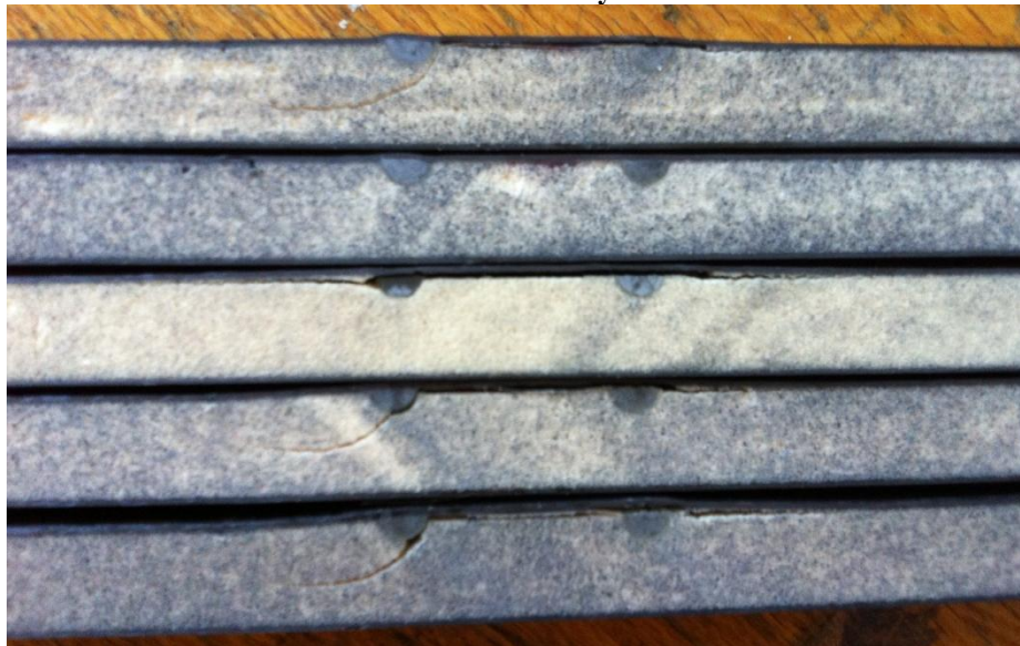
Figure 43. Final failure mode of control beam test group with one inch initial delamination and added transverse DAD keys.
