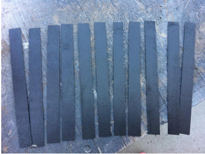
Figure 18. Test specimens cut using a tile saw
