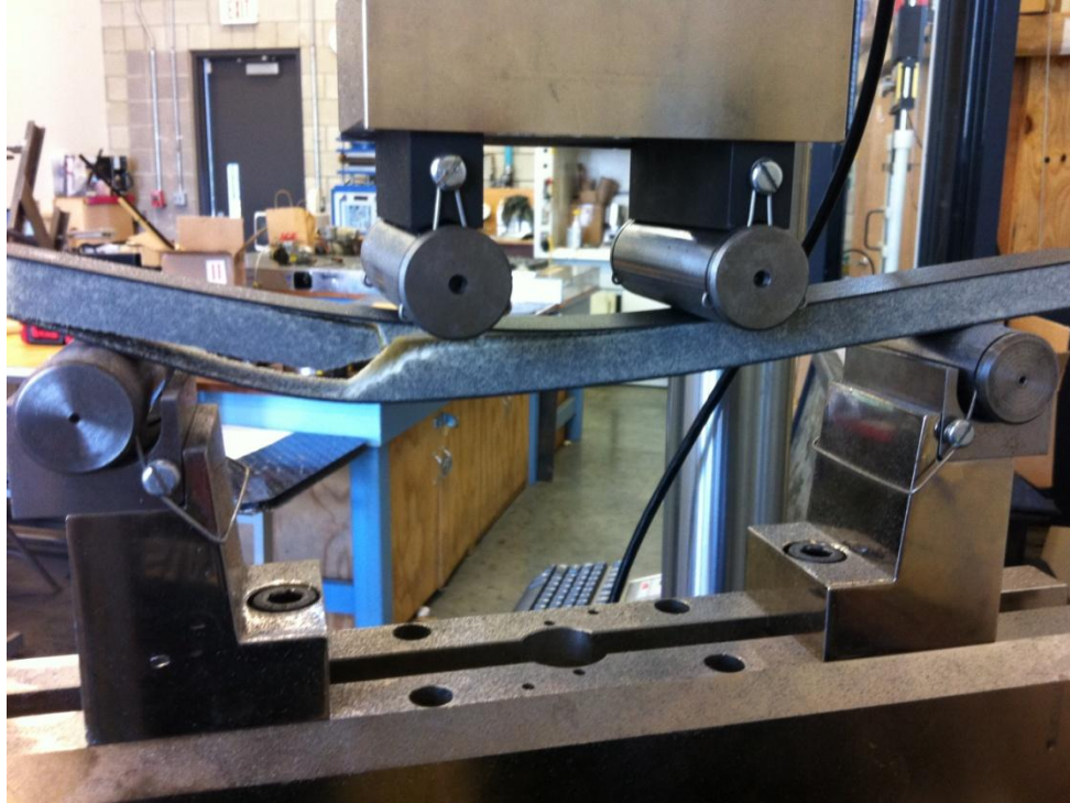
Figure 36. Typical failure mode of control case beam subjected to 4-point bending.
