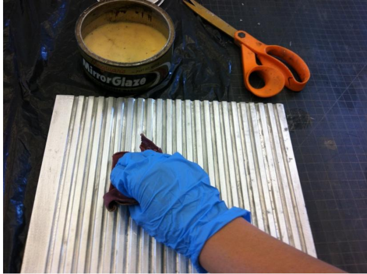
Figure 25. Mold release wax used to separate curved fiberglass from mold
