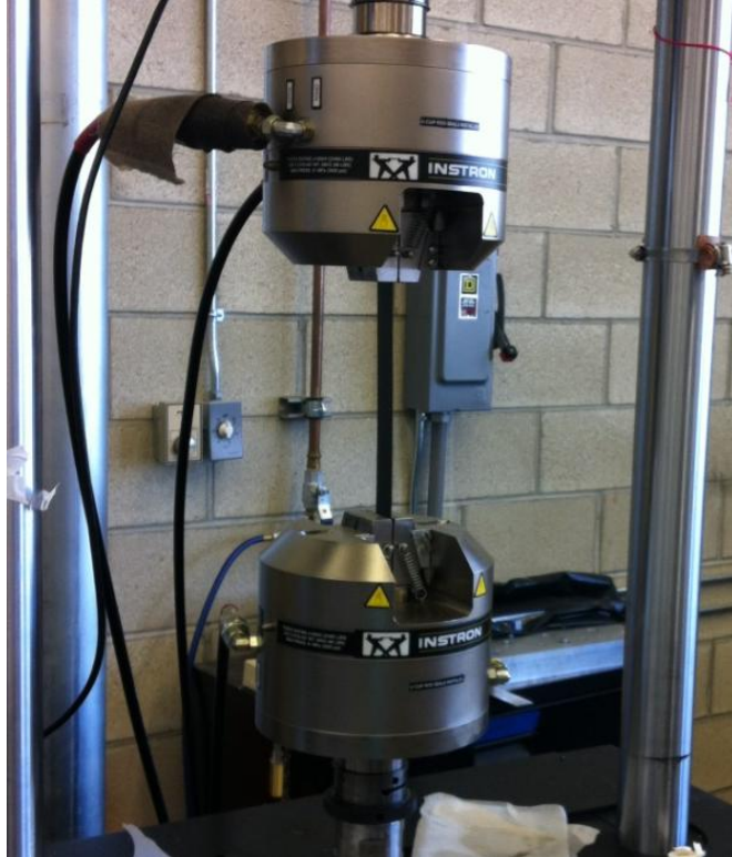
Figure 20. Carbon fiber test specimen placed in Instron 8801 test jig
