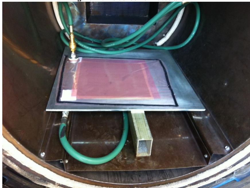
Figure 13. Part inside autoclave with hoses attached
