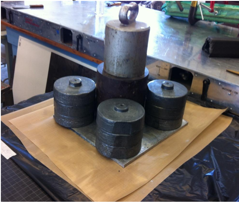
Figure 28. 200-lb of weight used to compress fiberglass DADs into mold
