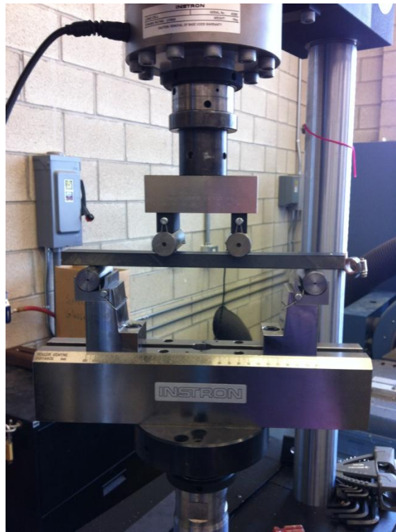
Figure 33. Instron 8801 Servohydraulic Fatigue Testing System used to apply four point loading on beams
