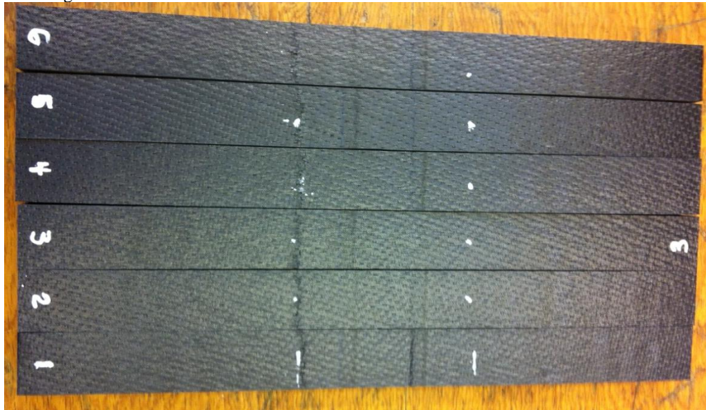
Figure 45. Final failure mode of control beam test group with added transverse DAD keys.
