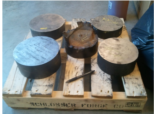
Figure 11: The five mandrel samples provided a total of 220 pounds of steel for further analysis. Fracture surface of a mandrel is in the center.
