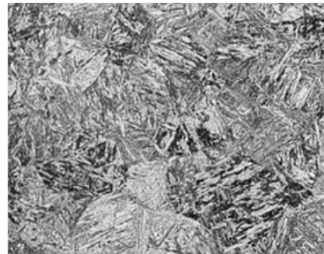
Figure 7: This micrograph is a mix of plate and lath martensite at 1000x magnification 10 .
