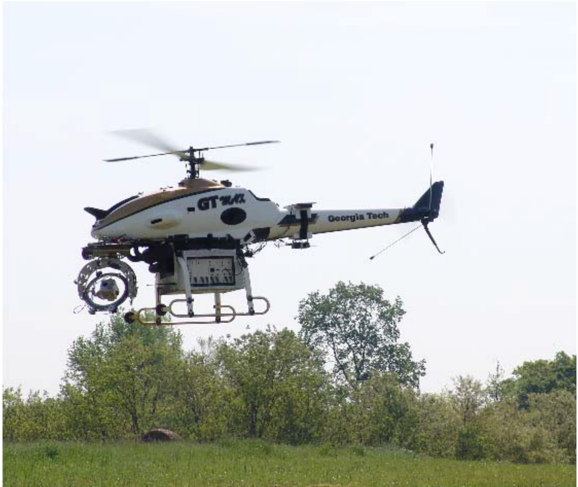
Figure 2-14 GIT 3axis gimbal on GTmax helicopter
