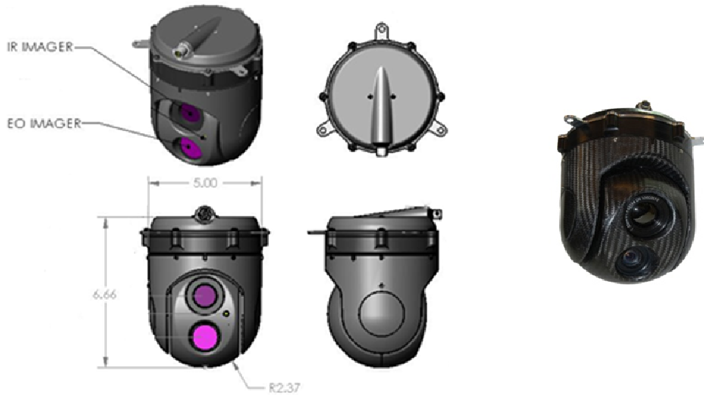
Figure 2-7 Tigereye dual imager 4-view & picture
