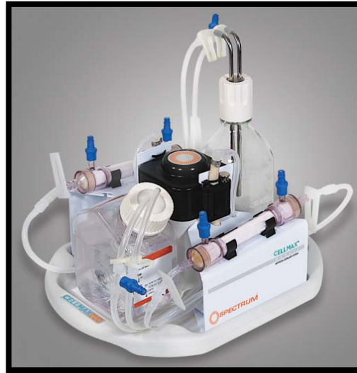
Figure 7: CellMax Duo Bioreactor system characterized by Bryan Brandon in the Cal Poly Tissue Engineering Lab [62].
