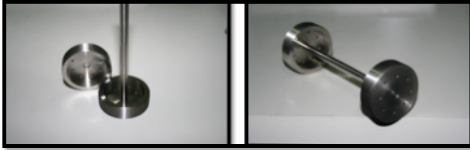
Figure 14: Machined scaffold caps with and without stabilization bar. Initial “dumbbell” configuration is achieved when insertion of stabilization bar into other scaffold cap.
