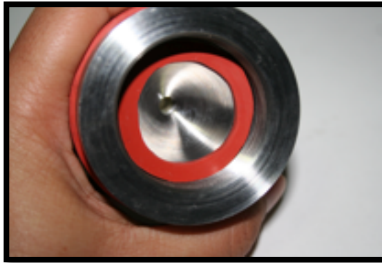
Figure 28: Custom internal O-ring used to seal inner contents of the bioreactor.
