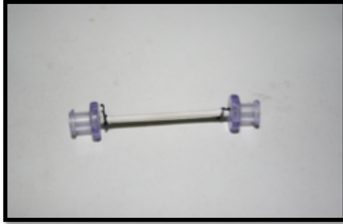
Figure 40: Scaffold sutured to two Qosina barbs ready to be installed into bioreactor.
