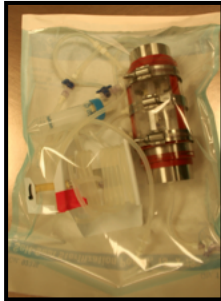
Figure 33: Bioreactor system packaged in one 13" x 18" sterilization pouch.
