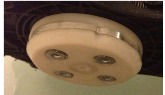
Figure 23. 3-piece machined cam attached to the bottom of a binding.
