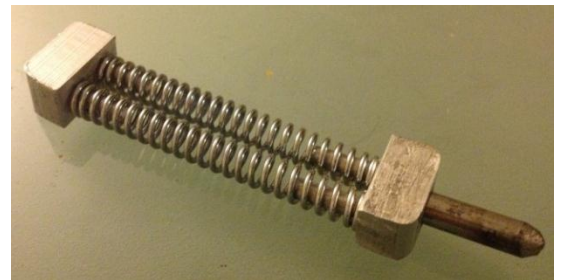
Figure 22. Final machined spring assembly with milled edges, press-fit aligners, and sanded follower tip.
