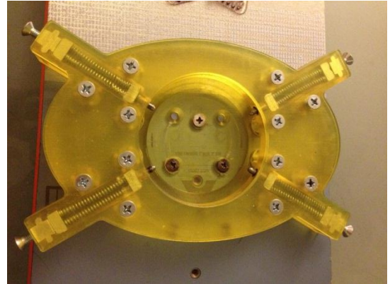
Figure 21. Final rapid prototyped baseplate with spring assembly.
