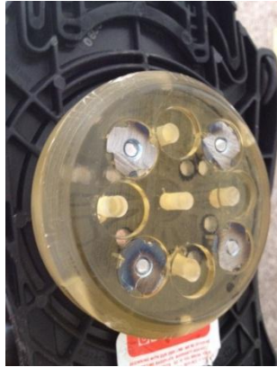
Figure 15. Initial Rapid Prototyped Cam Fixed to the Bottom of a Binding
