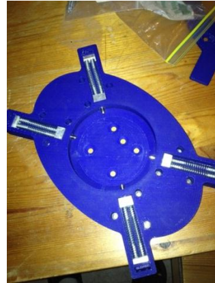
Figure 16. Initial Rapid Prototyped Baseplate with Springs, Followers, and Set Plates
