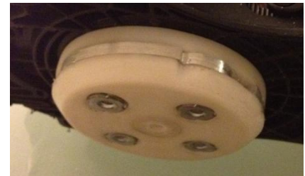
Figure 18. Final Machined 3-Piece Cam System with Notch.
