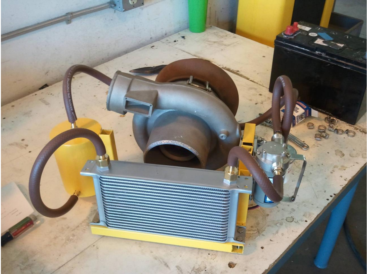
Figure 2-6: Oil System Subframe
