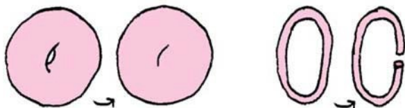
Fig. 9. Two ways of removing a handle, illustrated on two tori. The “fat” torus is best repaired by collapsing the handle, and the “skinny” torus is best repaired by pinching the handle.
