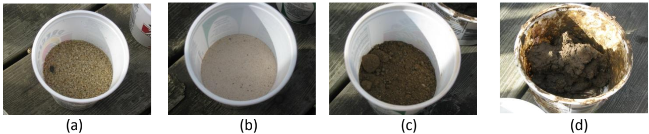
Fig. 2 Soil samples (a) coarse sand, (b) fine sand, (c) silty sand and (d) sandy clay
