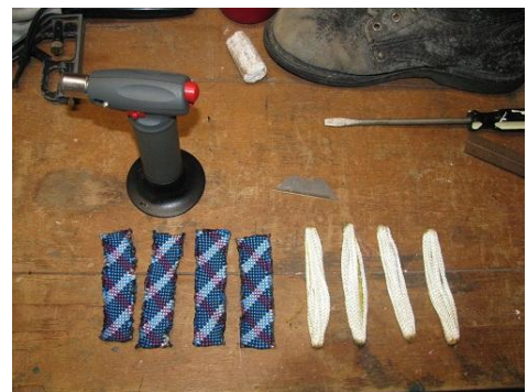
Fig. 4 Core separated from sheath and welded
