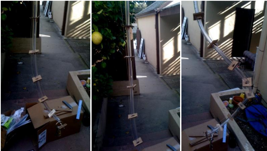
Figure 8 – From left to right: A) The un-actuated prototype with pre-set bend B) Prototype actuated against the pre-set bend curve C) Prototype actuated with the pre-set bend curve.
