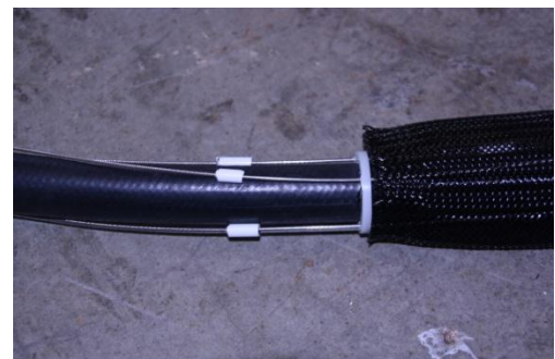
Figure 21 – Construction of Cable arm: rubber hose, cable guides, cable spacers, and actuation cables.
