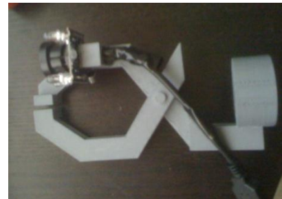
Figure 25 – Visual checks: detachable gripper, video and lighting capability.
