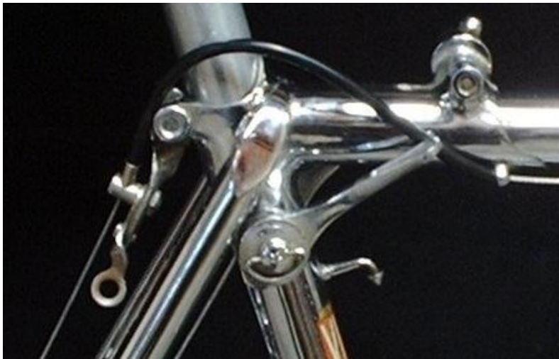
Figure 16 – Descriptive image of a standard bike brake cabling setup
