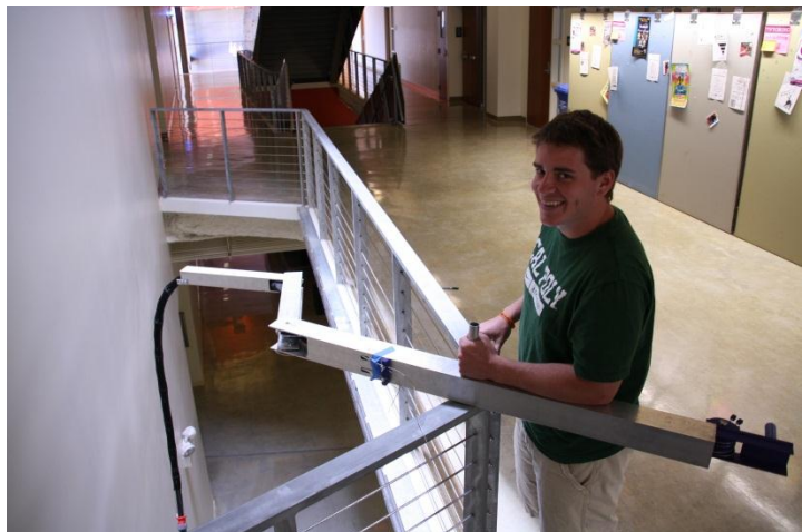
Figure 26 – Alex holding the prototype during testing. Cable arm draped over the end of the boom was able to actuate properly.
