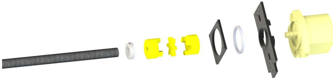
Figure 10: Exploded view of pump and pump cradle.
