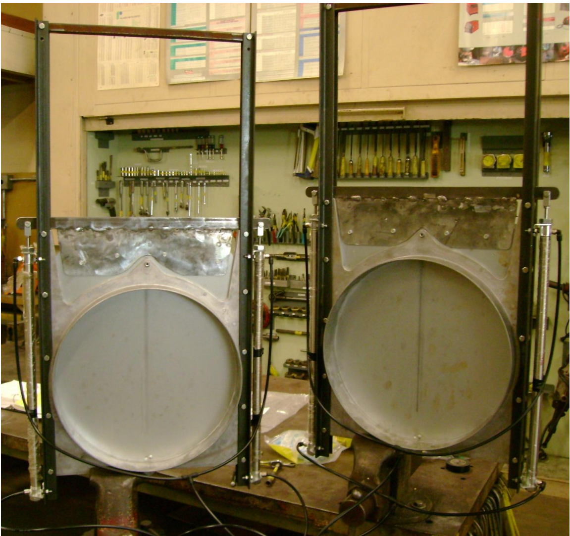
Figure 9. Blast gate valves.
