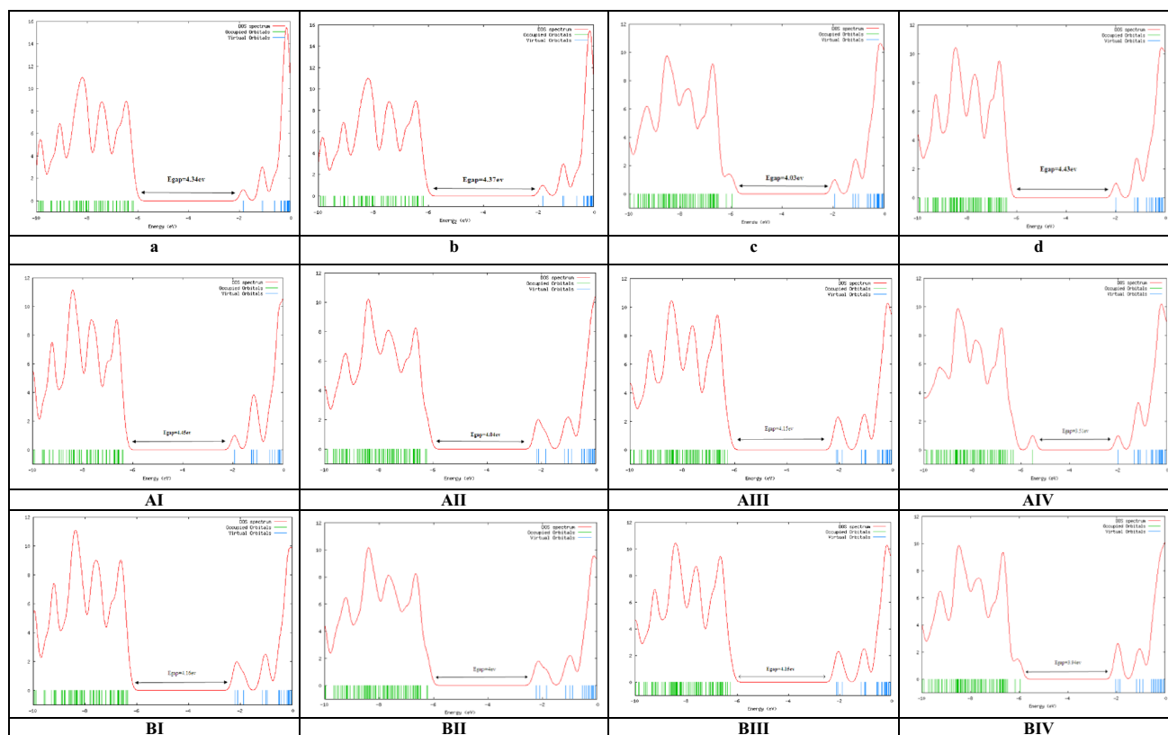
Fig. 5 DOS plot for adsorption CO gas on the surface of pristine and B, As, BAs-doped of (4, 4) armchair model of AlNNTs (models AI–BIV) and a–b unadsorbed models
