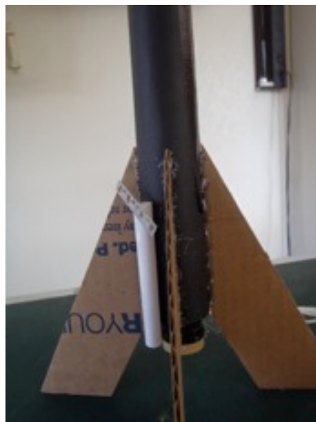
Figure 9. Straw and razor blade on test rocket.
