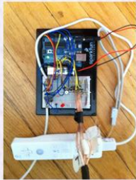
Figure 4. Our Arduino microcontroller plugged into a Wii remote. The accelerometer and buttons are all wired into the Arduino which acts as a Wii remote extension, similar to the nunchuk. This way, the Wii can communicate exclusively with the Wii remote.
