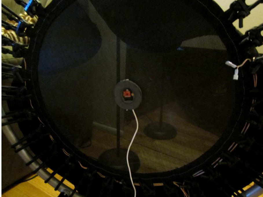
Figure 43. Mounted accelerometer with brass rods sewed into mat
