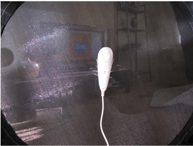
Figure 20. Close up of Wii Nunchuck attachment to trampoline
