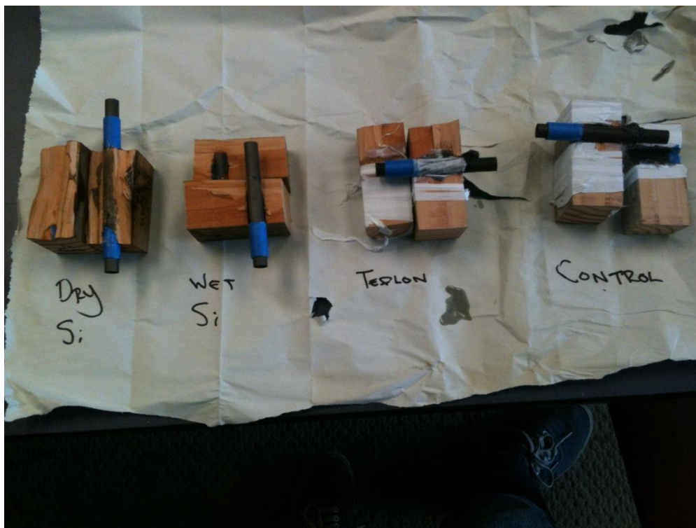
Figure 48-Experimental Joint release agents, using Dry Silicon, Wet Silicon, Teflon Tape, and a Control. All failed the test.
