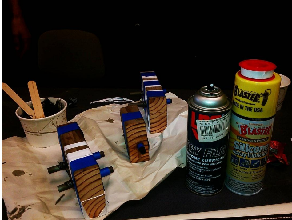
Figure 47-Joint test fixture and materials. This image is to be used as a reference not as a template for the test; the test follows the procedure specified in this document.
