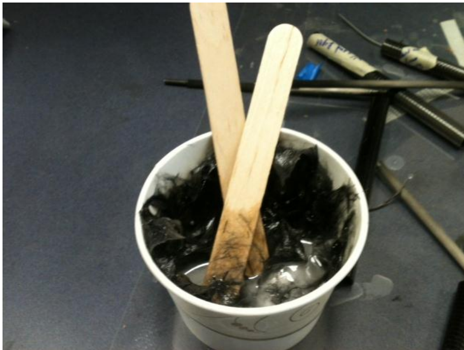
Figure 39: 1.2oz of Epoxy/Hardener mixture with 6" of epoxy.
