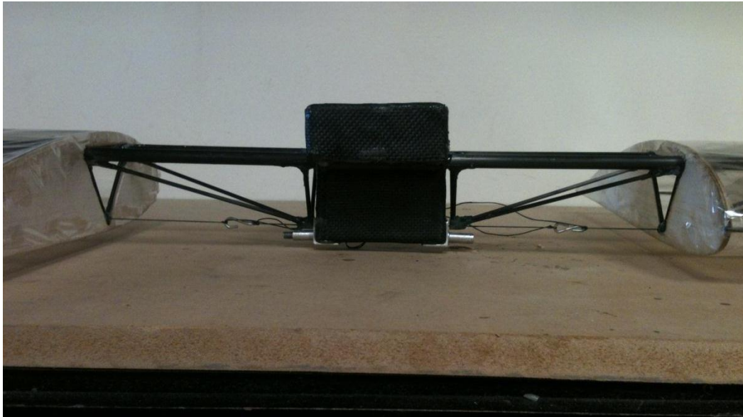
Figure 32-Installed Hub with Tension System
