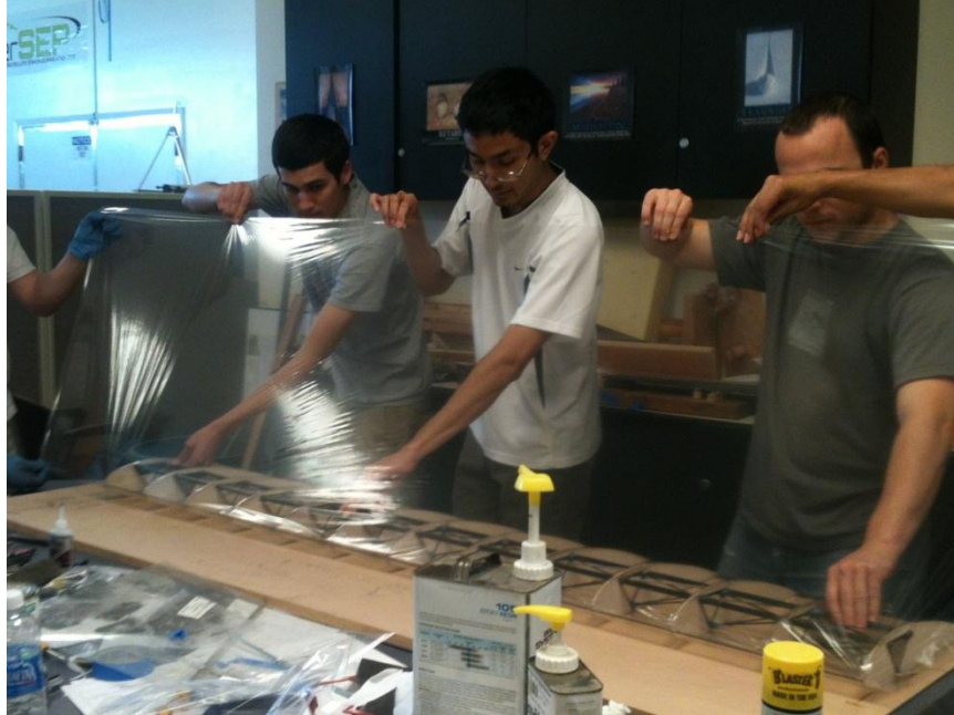
Figure 35-Installation of Mylar using second procedure, with help from Team Icarus.
