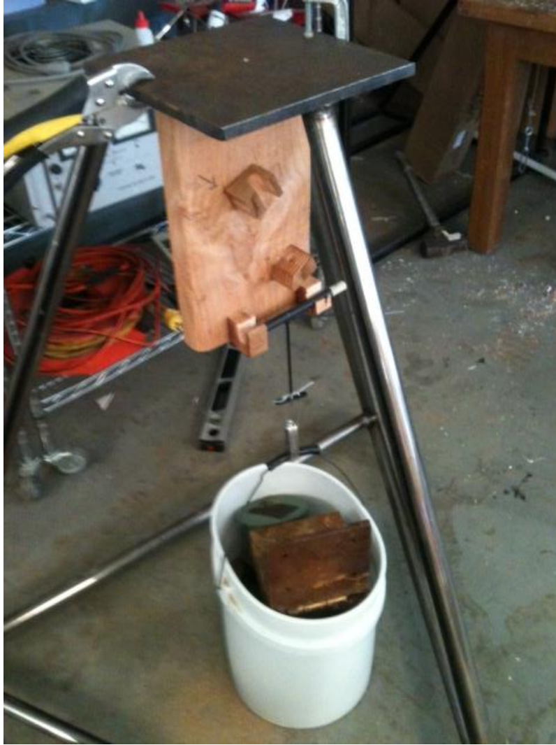
Figure 44: Test Fixture with loaded tubes, oriented in horizontal position. Bucket is filled with sand and known masses.
