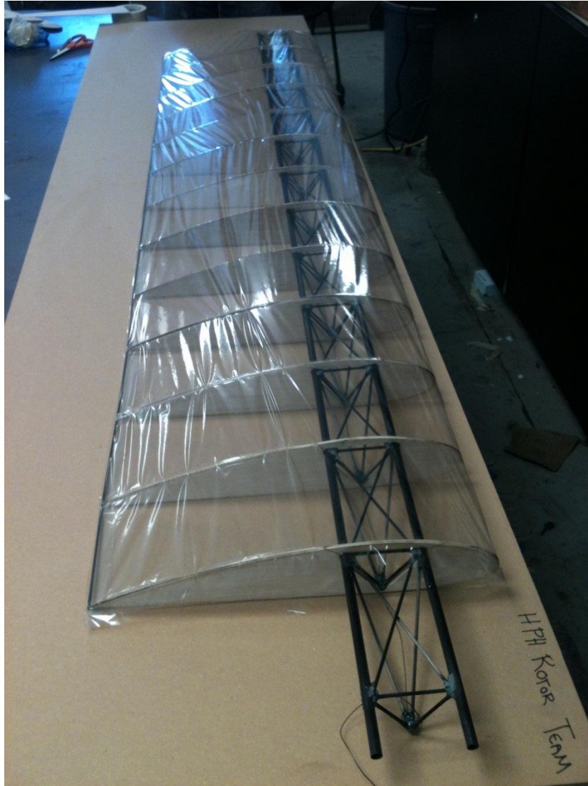
Figure 34-First Completed Wing using 1st Mylar Installation Procedure
