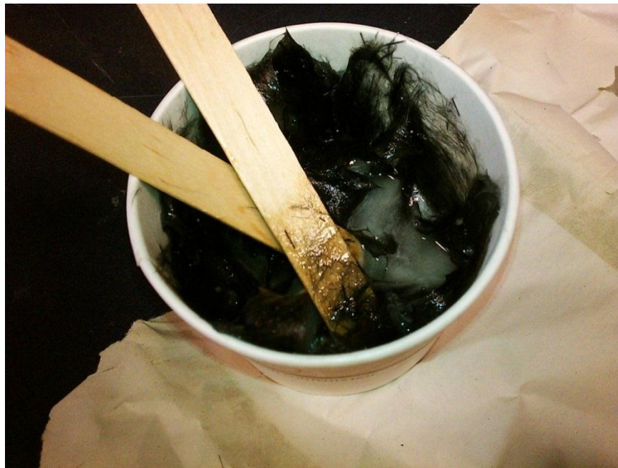
Figure 46-West Systems Resin/Hardener-tow mixture
