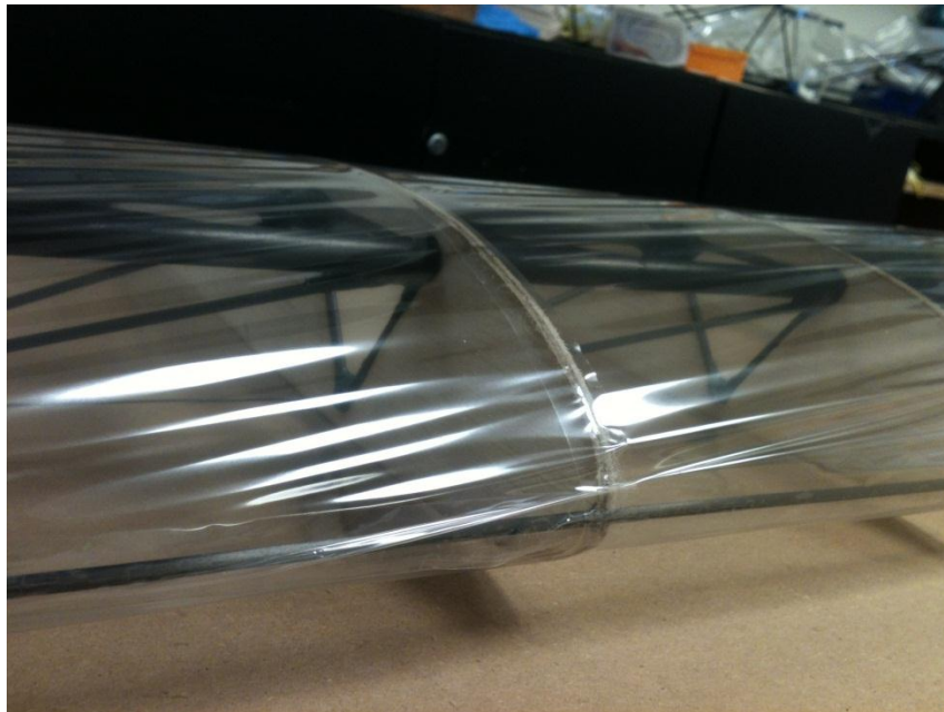
Figure 36-Finished wing from procedure 2. Note the wrinkles and leading edge.
