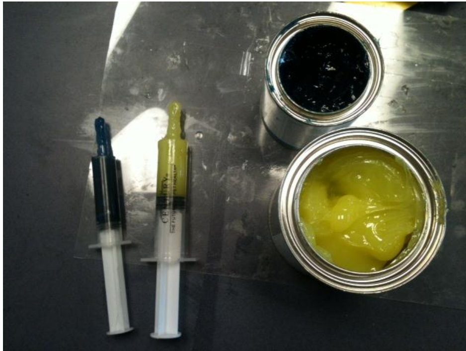
Figure 40: Pro-set Epoxy/Hardener with application syringes.
