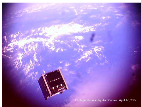
Figure 1.1: CP4 post-PPOD deployment - This image of CP4 was captured by Aerospace Corporation's AeroCube-2 CubeSat shortly after P-POD deployment.
