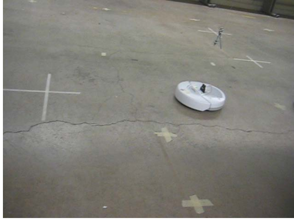
Figure 6.9: Particle Filter Test: iRobot® Create moving toward location of known distance (tape).
