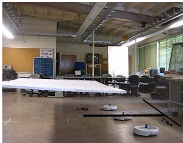
Figure 6.1: Experiment setup: Three iRobot® Create before navigating under a simulated ice edge with global axes displayed.
