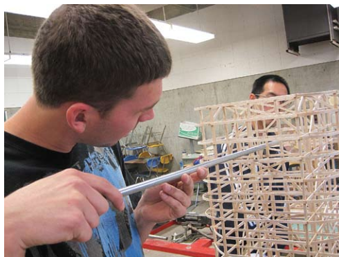
James Myers tests the width of the weight connections where the simulated live load will be placed for competition.
