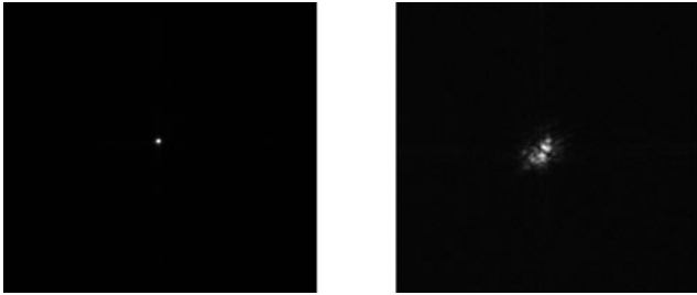
Fig. 11 Acquisitions of a pointlike source with the Fresnel Imager. Most of time we could see images close to left picture, but we also sometimes had to deal with unexpected air turbulence, as can be seen on right figure, showing a ‘nice’ speckle pattern
