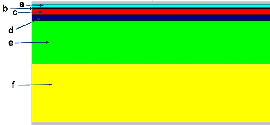
Figure 4 Conventional LED ; a) p-GaN, b) MQWs, c) n-GaN, d) \text{Al}_x\text{Ga}_{1-x}\text{N} , e) GaN buffer, f) Sapphire
