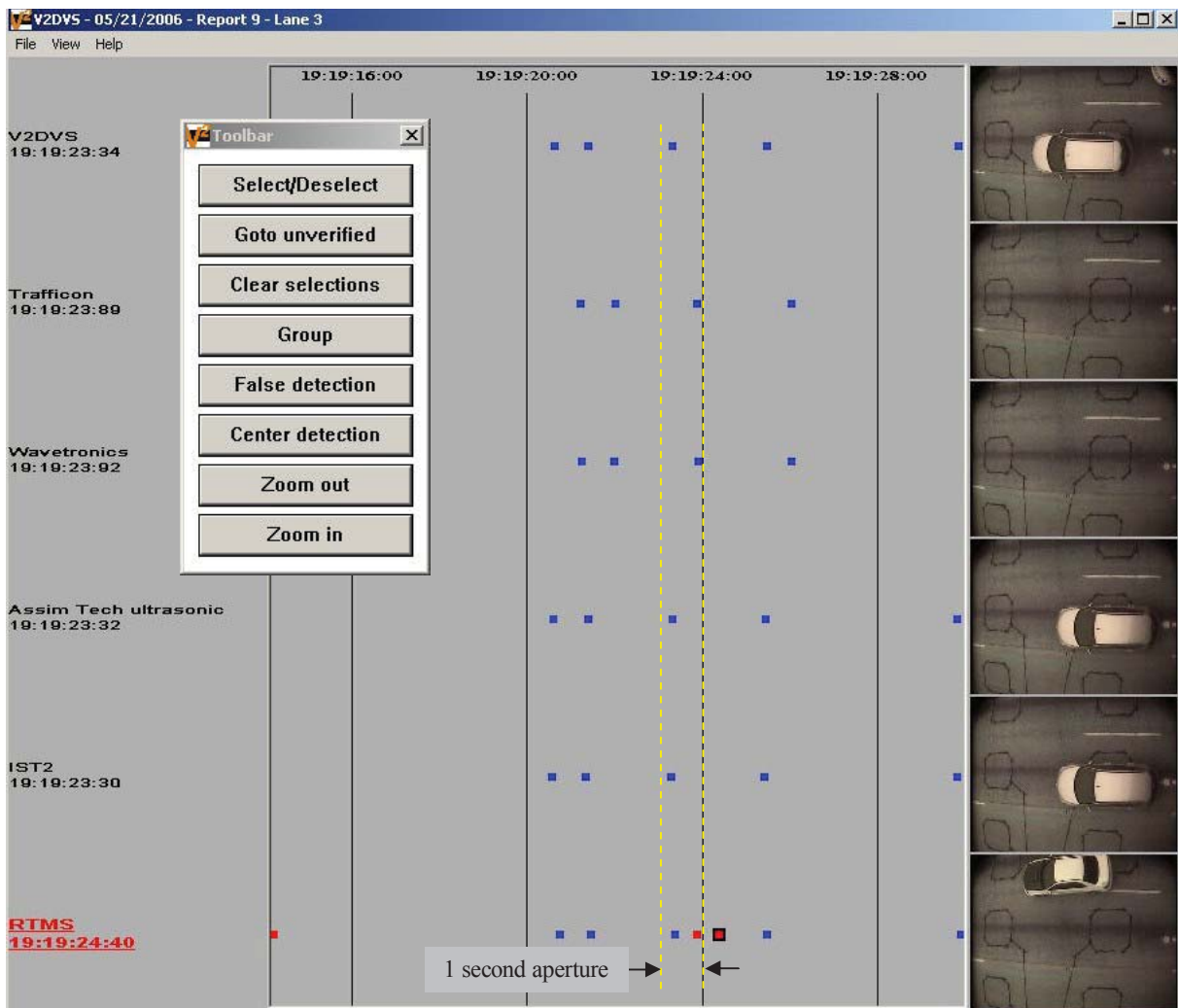
Figure 7. Manual verification window, showing the position-corrected time line for each detector. The correlation aperture for a selected vehicle is overlaid. Automatically correlated detections are blue dots. For the sixth detector, the automatic designation of two false detections is shown by red dots. For the second and third detectors, the detection position was outside camera view.
