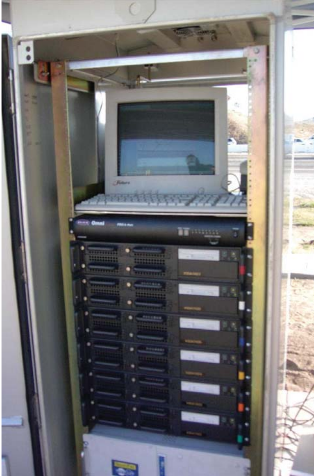
Figure 1. V2DVS field computers in Type 334 cabinet.
