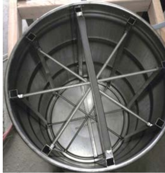
Figure III-6. Plenum internal structure.
