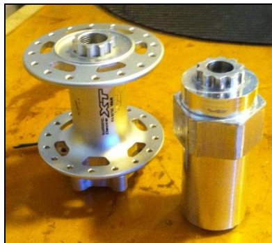
Figure 26. Custom hub design side-by-side with a standard bicycle hub
