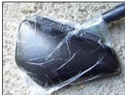
Figure 14. A crude but effective vacuum bag
