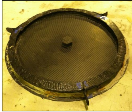
Figure 24. Carbon fiber disc mold with 3-piece rim mold attached and aligned
