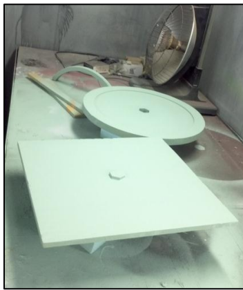
Figure 19. 3-foam mold pieces coated in a first layer of Duratec
