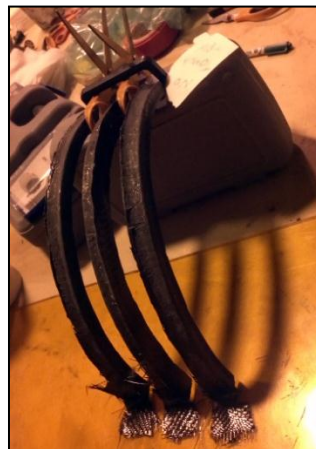
Figure 22. Flanges drying on hoop pieces after hand layup
