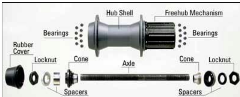
Figure 7. Cup and Cone Type Freehub
