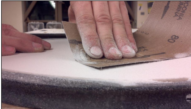
Figure 28. Sanding down the foam core before gluing the flat disc on
