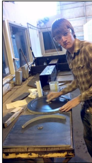
Figure 20. Applying Frekote to mold surfaces
