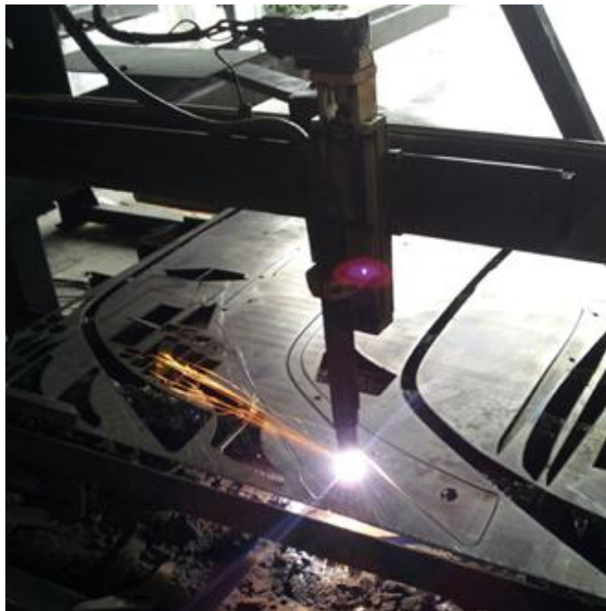
Figure 24: Plasma Cutting Unformed Brackets
