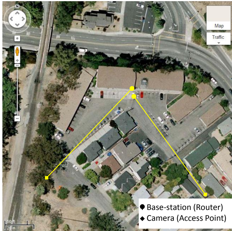
Figure 33: Range testing with omnidirectional antenna over 802.11n
