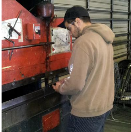
Figure 25: Press Brake Used to Form Brackets
