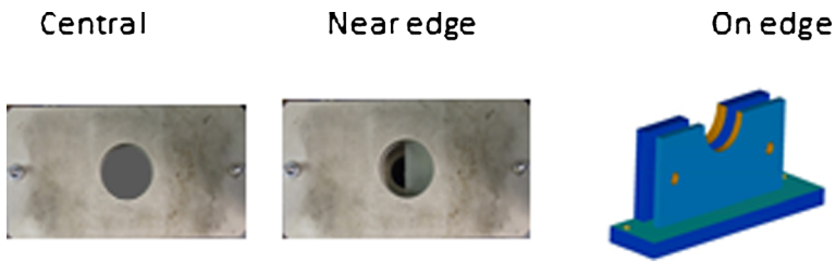
Fig. 2 Boundary conditions for the impact tests
