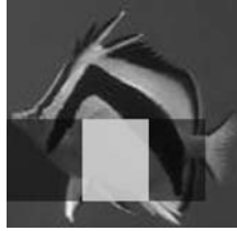
Figure 2. Example of a 2-rectangle Haar-like feature used for detection of the Scythe Butterfly fish
