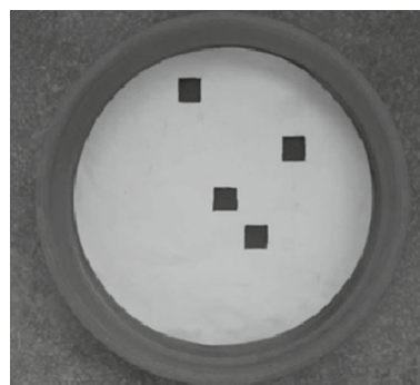
Fig. 4 Control sieve with a template used for calculating the screen blocking coefficient
