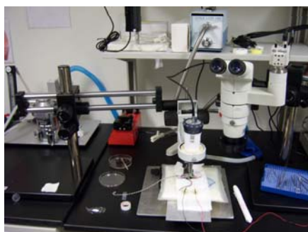
Figure 2. Intravital microscopy imaging station for functional vasodilation measurements.
