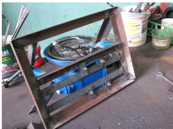
Electric pump bolted on the “tracks”
