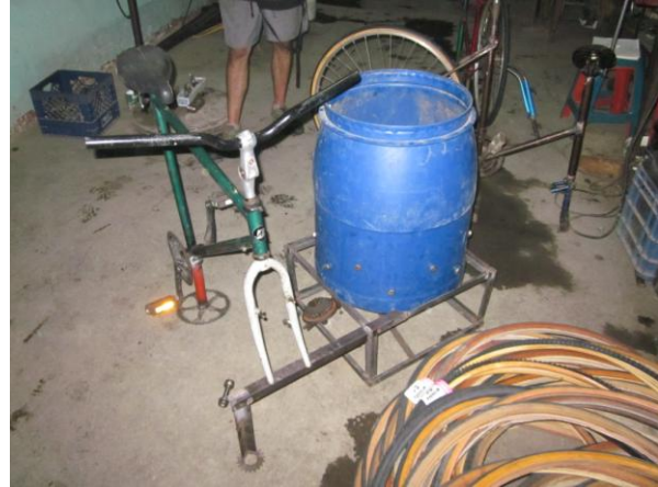
Initial prototype for a chicken-defeatherer
