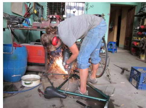
The painted stand (left). Cutting an old bike frame to use the parts for a bike machine (right).
