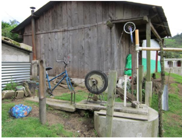
A Bici-Bomba used at a local farm
