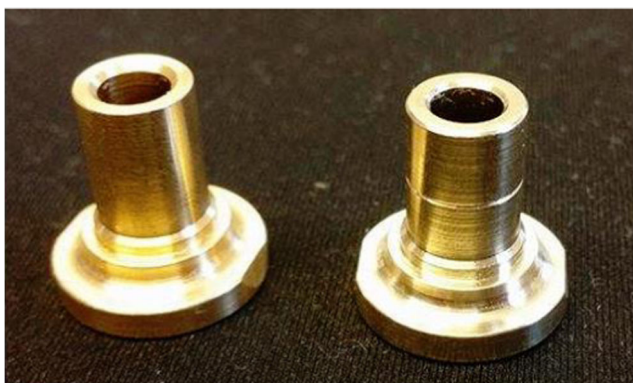
Fig. 6 Examples of the roughly 20 mm long socket. The left socket is produced in CuZn39Pb3 and the right in CuZn21Si3P
