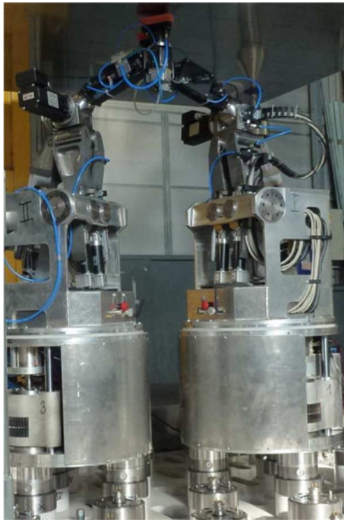
Fig. 1 Two cooperating mobile agents supporting a workpiece in the SwarmItFIX project
