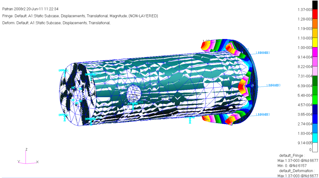
Figure 7: Patran/Nastran numerical calculation of the deflection due to the bolt load and indicate that there will be no problems from the bolts flexing.
