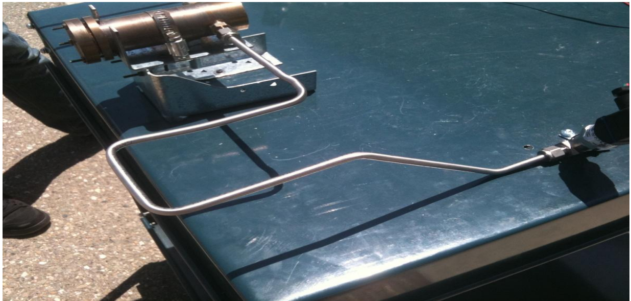
Figure 12: This picture shows the bend put into the pipe to allow the thruster to rotate on it's hinge. The other side mirrors the side shown.
