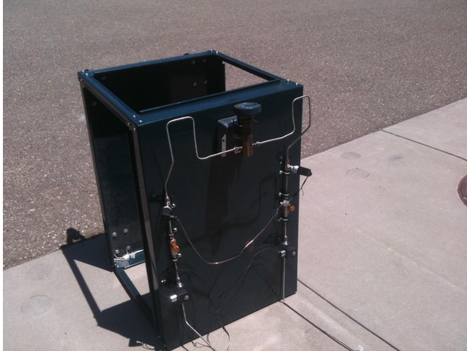
Figure 19: This picture shows the test apparatus tilted on it's end with a weight on the thruster for load cell calibration.
