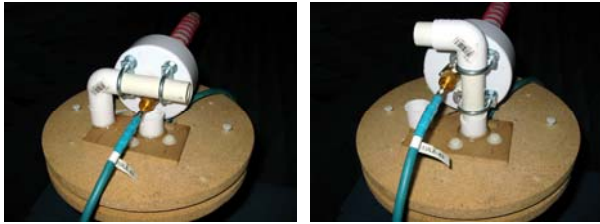
Fig. 4 Mounting of a Circularly Polarized Helical Antenna: Horizontal and Vertical Orientations
