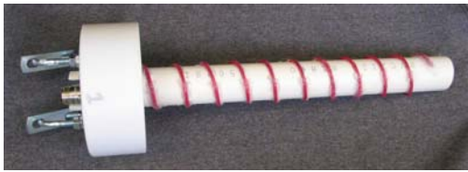
Fig. 12 Helical Antenna on Coil Form and End Cap Ground Plane
