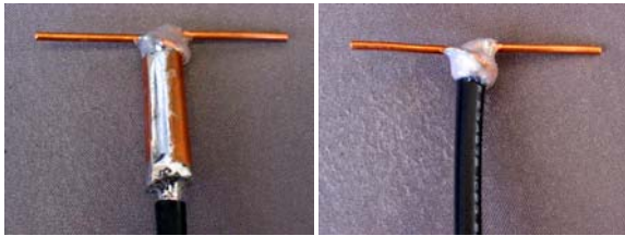
Fig. 9 Dipole with and without Sleeve Balun
