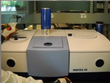
Infrared spectrometer, modified for emissions
