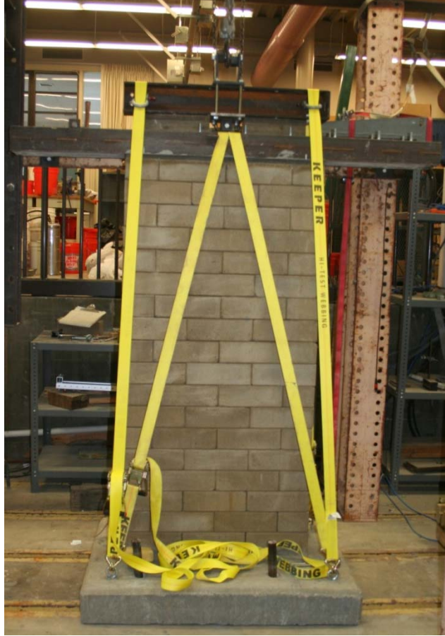
Figure 5-1: W4 being lifted into place with a crane
