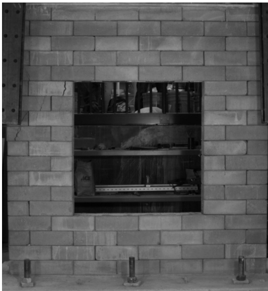
Figure 6-53: Cracking pattern of W6 prior to Cycle 21
