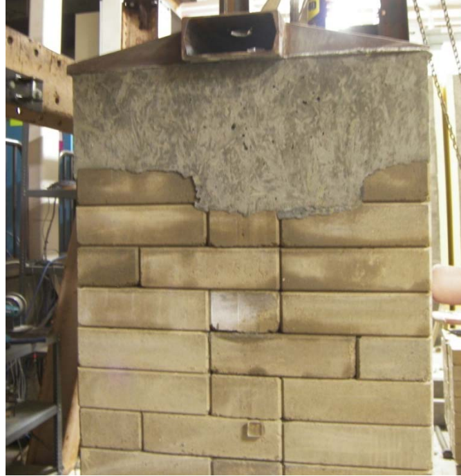
Figure 6-24: Flange of W5 after removal of the reinforced concrete formwork
