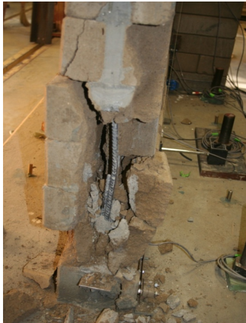
Figure 6-36: Spalling of the ICEBs and grout around the toe of W5 web
