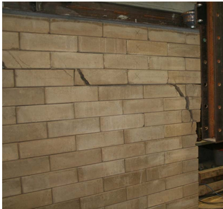
Figure 6-18: Damages in W5 Web resulting from mechanical failure of actuator
