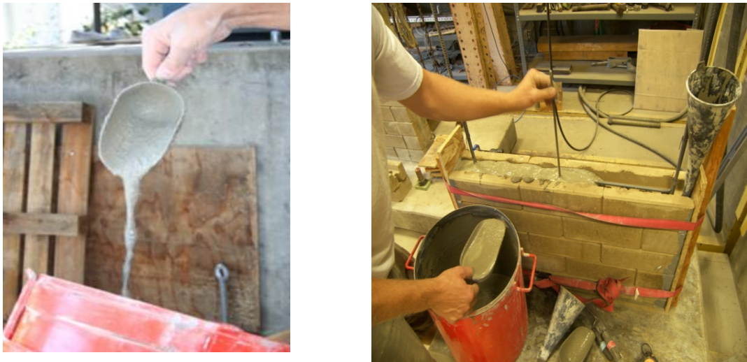
Figure 4-5: Grout used in specimen construction
