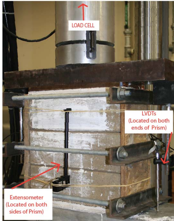
Figure 3-3: Masonry prism test setup
