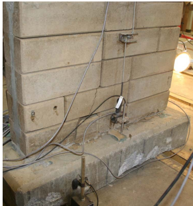
Figure 6-40: Cracking at the base of the flange of W5
