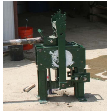
Figure 1-2: Soeng Thai BP6 Block press
