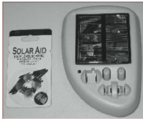
Figure 4: Godisa solar powered battery recharger. (McPherson, Brouillette 2004)
