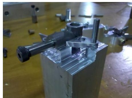
Figure 18: Knuckle Welding Fixture
