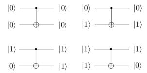
If the control and target qubit were swapped, then the CNOT gate would appear upsidedown relative to how it was previously shown and perform accordingly.
