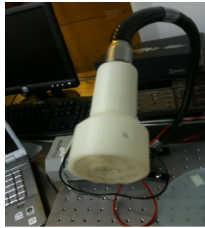
Figure 8: Photograph of the ABS fitting for integrating the lens with the Fiber-lite system.
