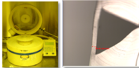
: Laurell Technologies 400WX spin coater al Microscopy Image of Film Thickness
