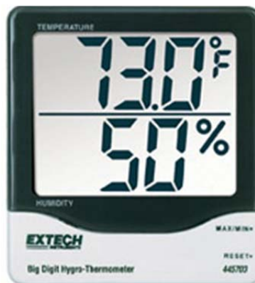
Figure 33. Hygro-Thermometer measures relative humidity within +/- 5%
