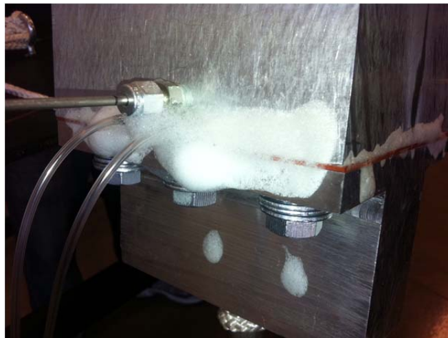
Figure 55. Soap was used at the gasket seams and pipe connections to test for leaks
