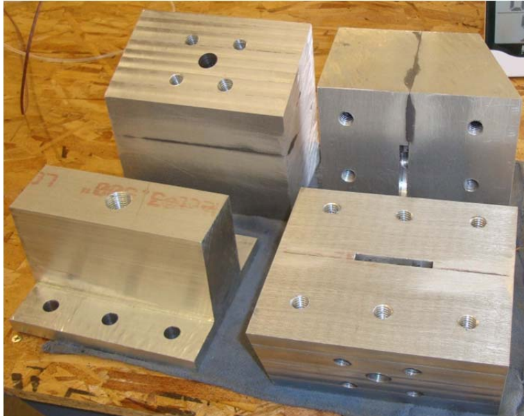
Figure 51. The transition piece and three test blocks required over 200 hours of manual machine time
