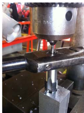
Figure 50. Thread tapping was completed with care using a tap guide
