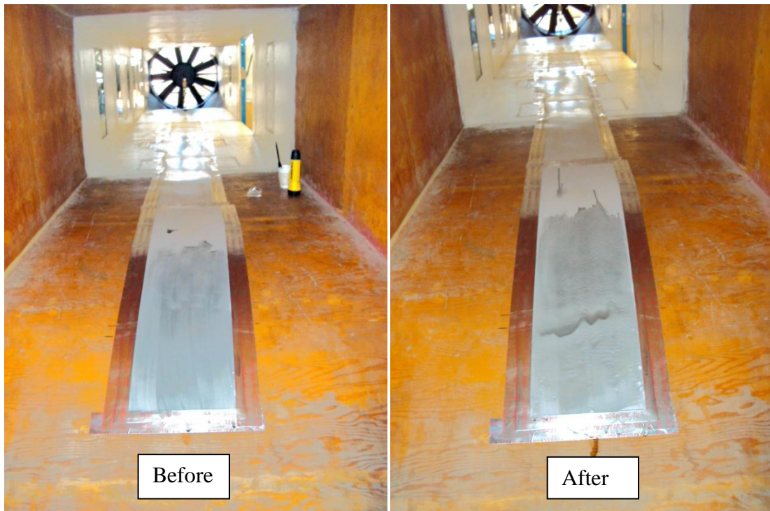
Figure 50 Flow visualization showing oil pooling in the throat (before and after)
