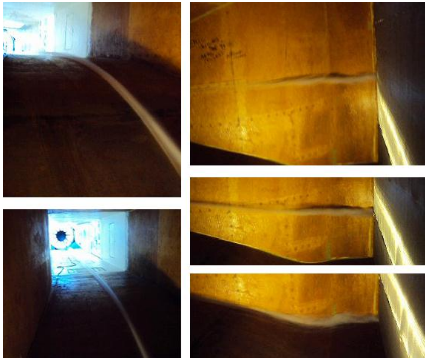
Figure 59 Streaklines after screen and honeycomb replacement
