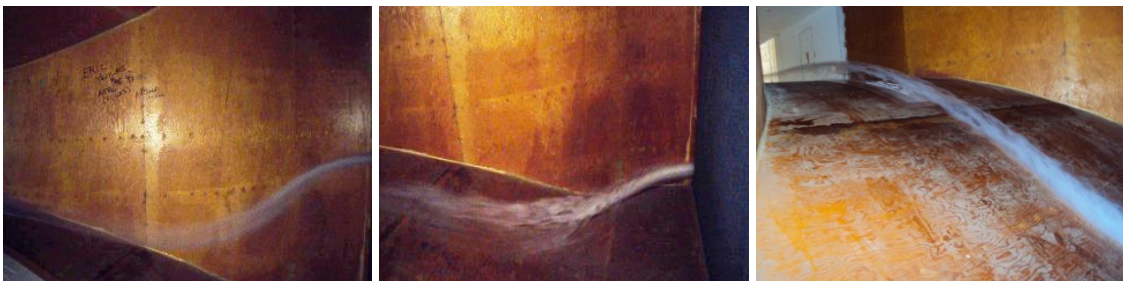
Figure 49 Smoke visualization inside the inlet
