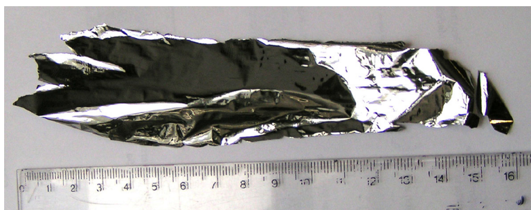
Fig. 10 The 4.5–5.5 μm foil of 3 cm × 15 cm produced from natural Mo
