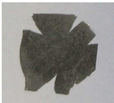
Fig. 7 The 80\ \mu\text{m} thick foil produced from the droplet obtained by melting the Mo pellet beforehand sintered at 1\ 600\ ^\circ\text{C} under the hydrogen atmosphere
