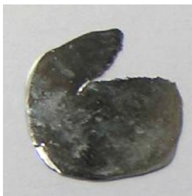
Fig. 9 nat Mo after hot flattening and cold rolling down to 320 μm
