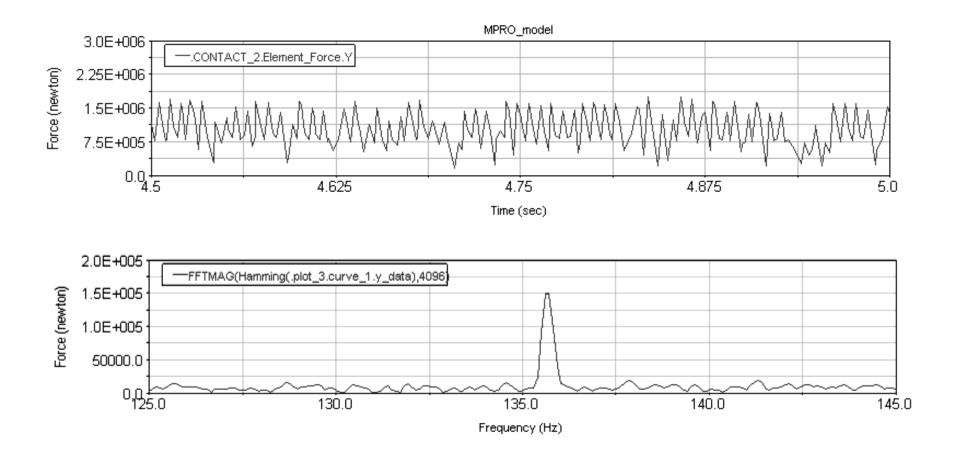
From the contact forces, we can get the meshing frequencies by FFT.
