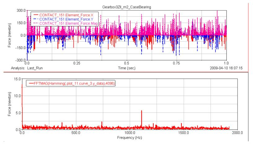
The peaks in FFT plot shows the meshing frequencies and meshing stiffness frequencies.
