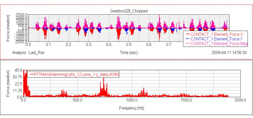
The FFT for the contact force shows the modulated side bands because of tooth malfunction.
