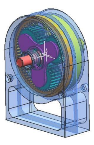
This is a 3ZII type planetary gearbox with large gear ratio. Here is a scaled model with module 2 and gear ratio 134.
