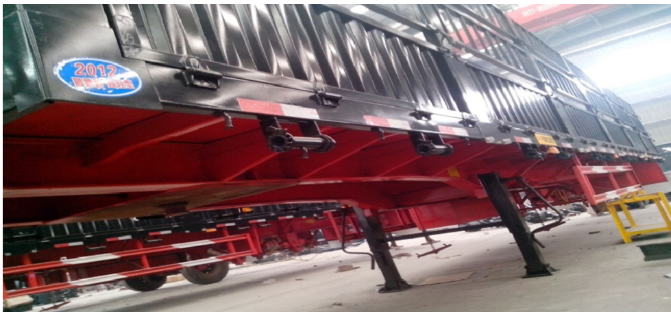
Fig. 6 Lightweight semi-trailer made in China by high strength steels with yield strength above 900 MPa
