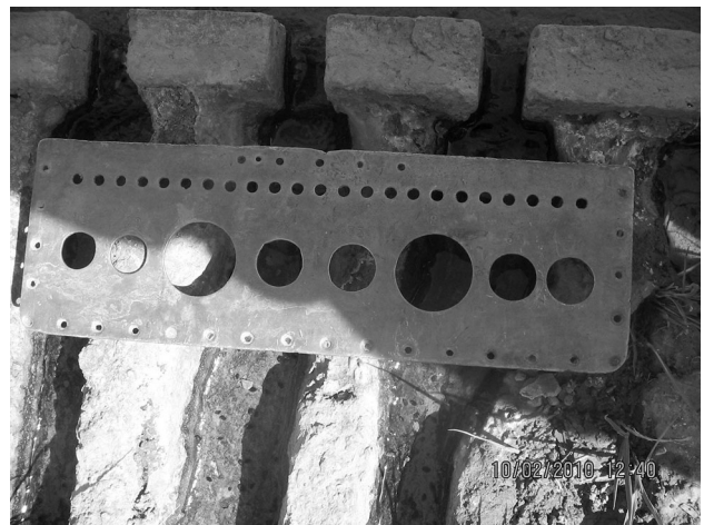
Fig. 8 Gauging plate (Louh) used in the oasis of Timimoun
